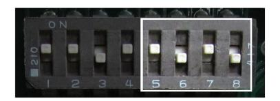
Peel this corner back to access dip switches.
